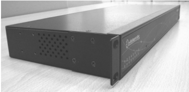
Installed L bracket:
