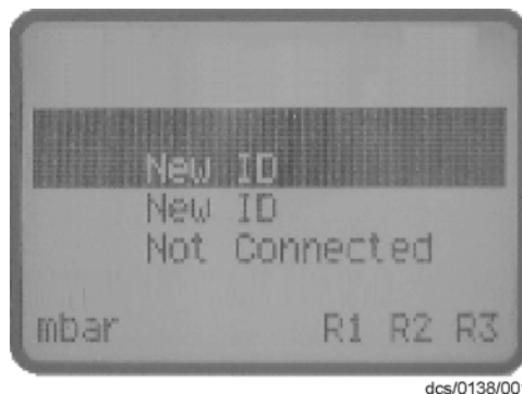
Figure 16 - New gauge connected
