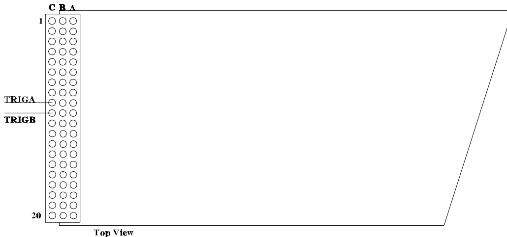
Figure 7 M321 M-module connector orientation
