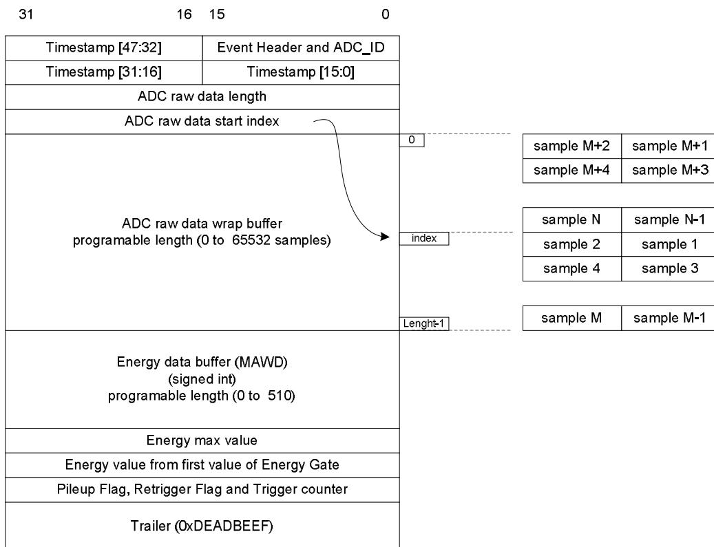
Two 32-bit words are added to the Event Buffer: “ADC raw data length” and “ADC raw data start index“.
